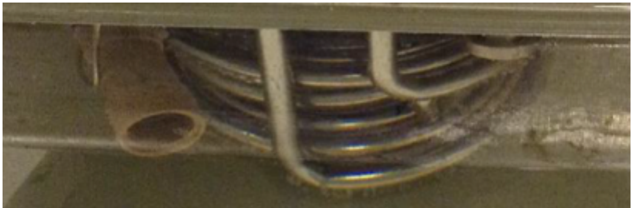
Figure 10a. Heating element in heating bath with water on Day 1.
