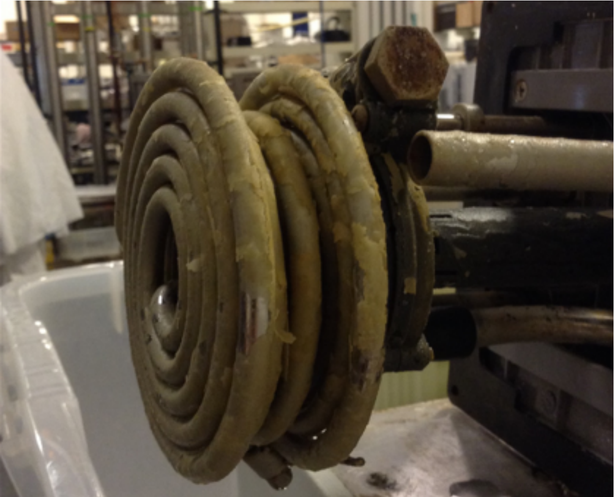
Figure 11a. Heating element with deposited solids after test run with Chemfree technology. Clear spots on the stainless steel element are present and the solids were not chemically bound to the element.
