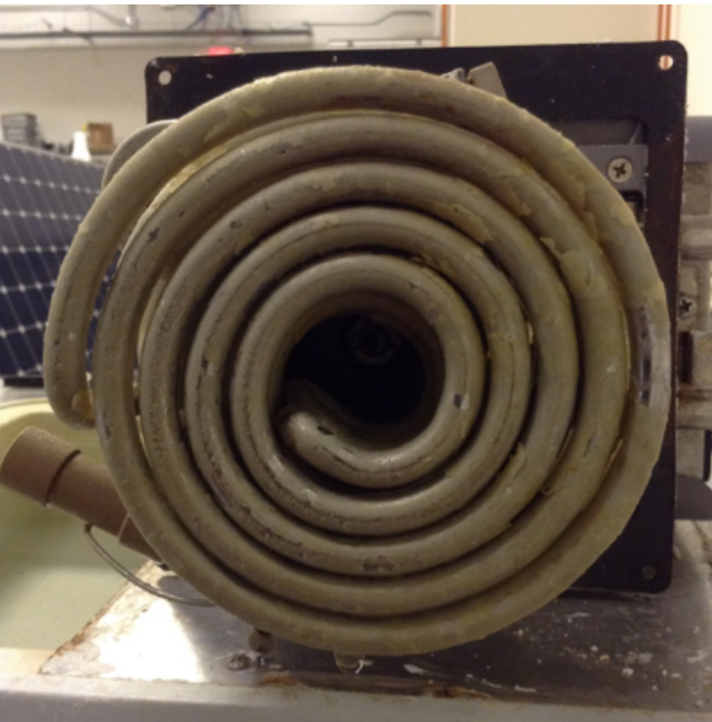
Figure 11b. The bottom of the heating element after testing with Chemfree technology. The bottom of the element has many clear spots which is consistent with deposition of solids as compared to scale formation directly on the element. The element was easily cleaned with physical brushing and did not require acid washing.
